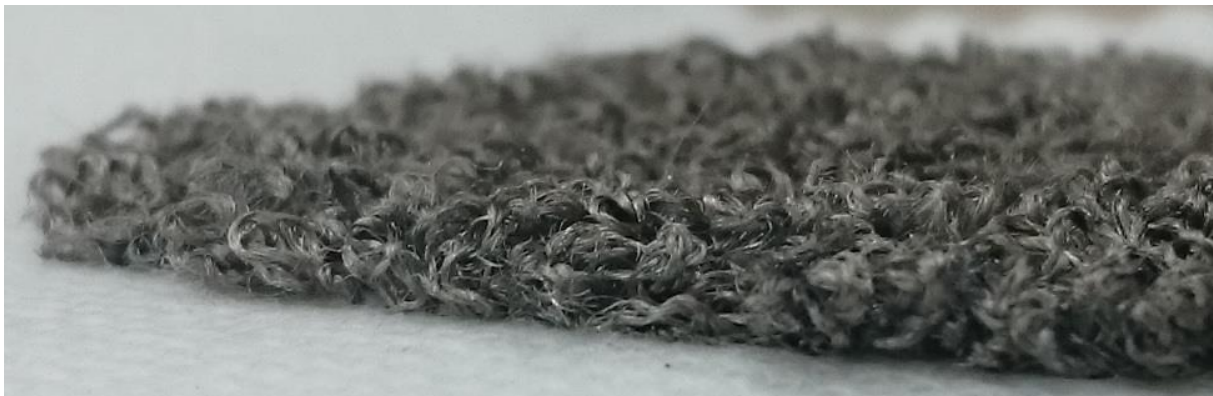
Figure 3 3D-structure of a moss-embroidered electrode
