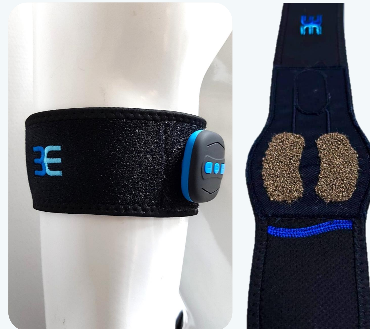
EMS wearable with moss-embroidered textile electrodes by 3E
